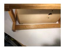
Two holes on the bottom should line up with the pins on the frame
