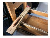
Each key slides onto a metal pin at the top and bottom
