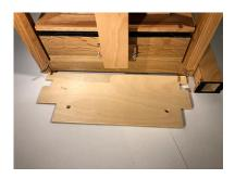
The other side of the plate has notches for the legs of the frame.
