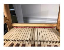
Slide the small crossbar onto the tall pins, tapered side down. Don't forget to match the numbers!
