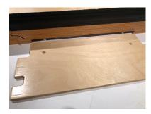
Two pins on the bottom of the bellows fit into those hole.
